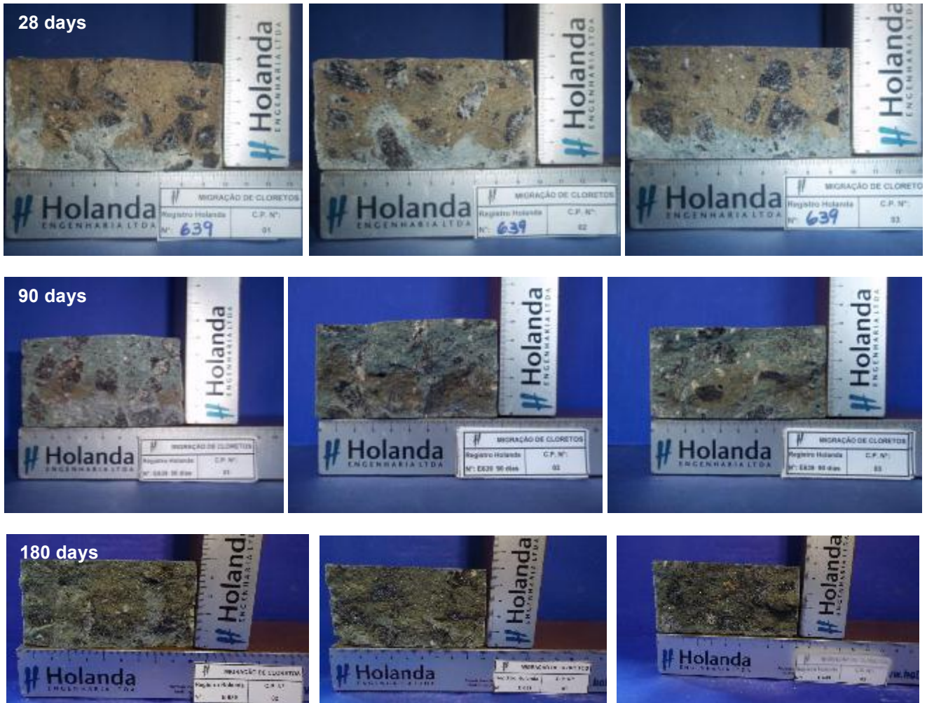
Figure 1: Depths of chloride Penetration at 28, 90 and 180 days – EXP 639 (0,0% Admix).
